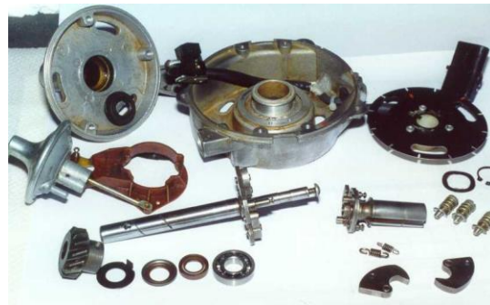
Figure 3 Richard Dowlings distributor, completely disassembled.
