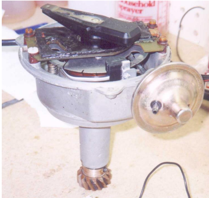
Figure 8 Distributor assembled with Crane ignition.
