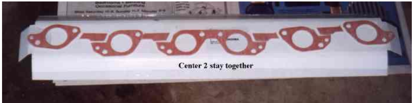
Figure 6 Cutting intake manifold gaskets.
