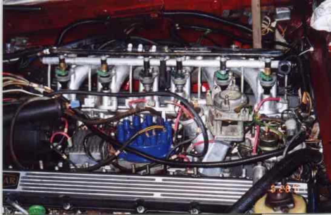
Figure 7 Installing right intake manifold.
