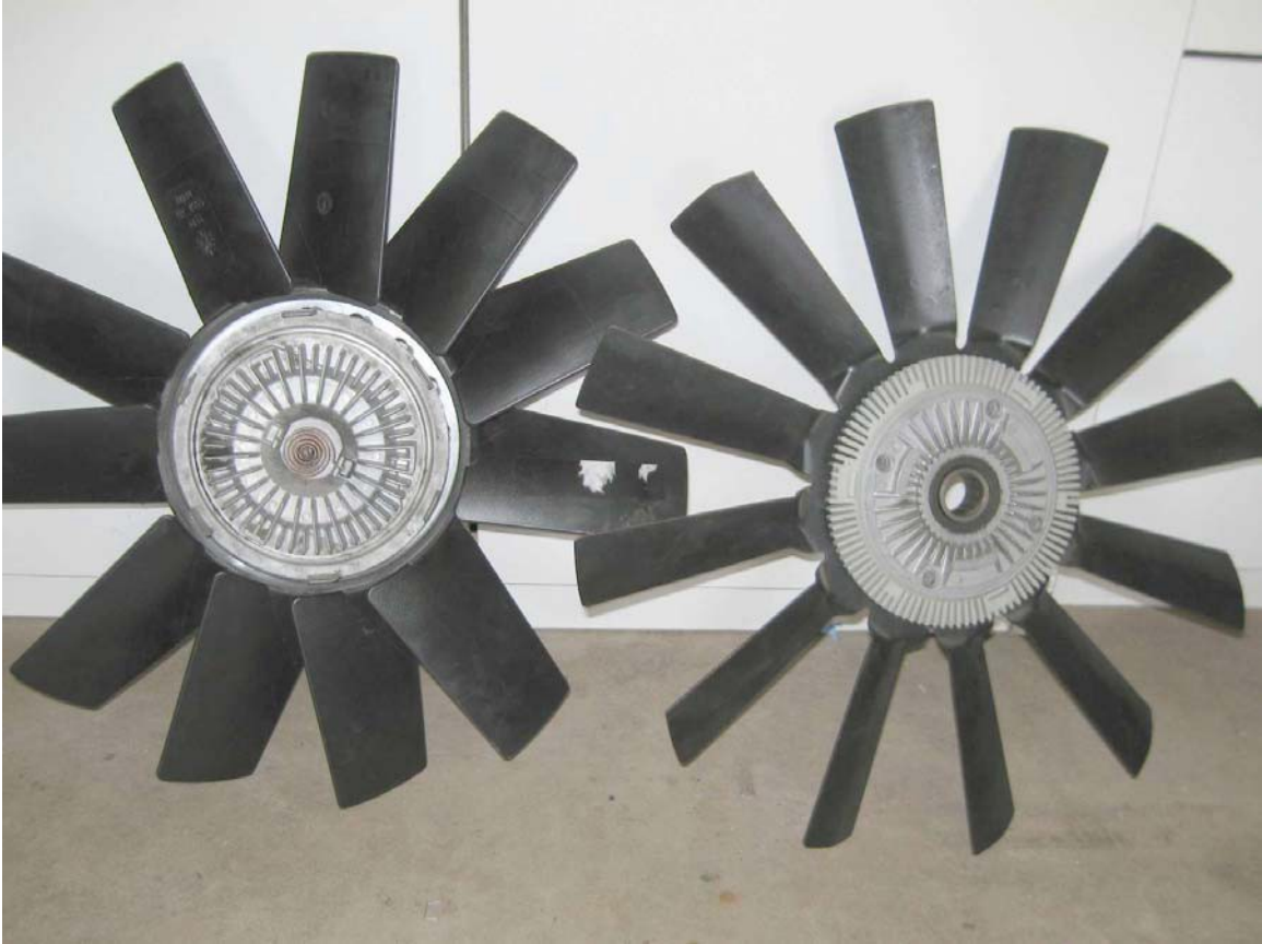
Figure 1 HE (left) vs. preHE fans and clutches
