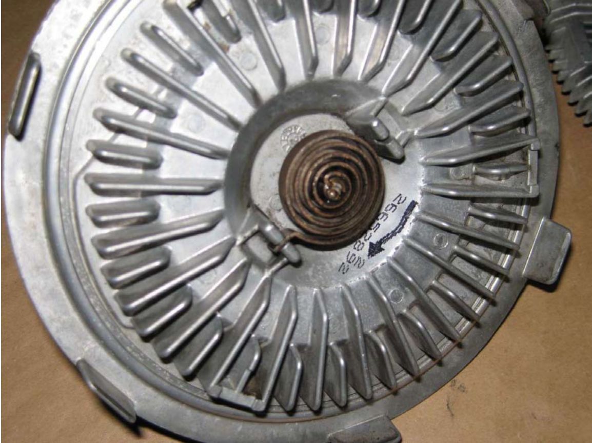
Figure 3 Thermostatic element on HE clutch.
