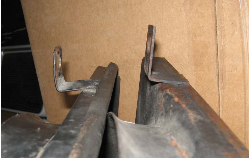
Figure 7 HE (left) and preHE (right) fan shroud difference.
