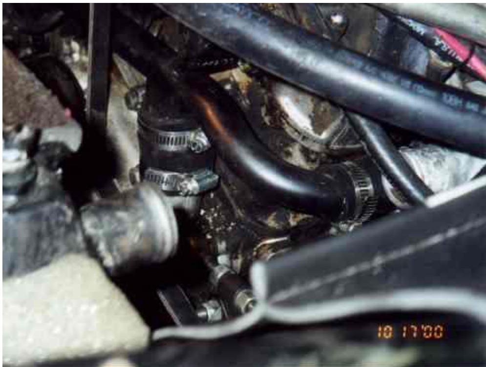
Figure 1. Crossover connections at left side and water pump.
