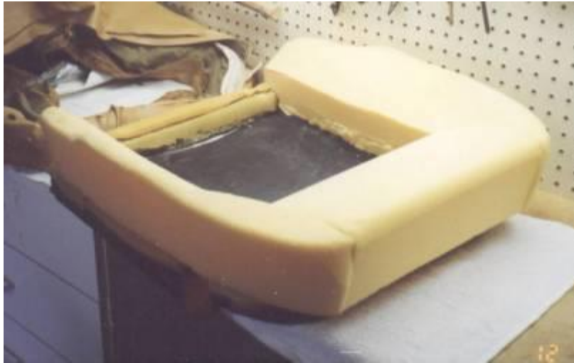
Figure 3 Bolster attached to frame.
