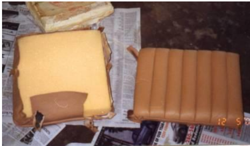
Figure 5 Replacing foam pad in center chshion.
