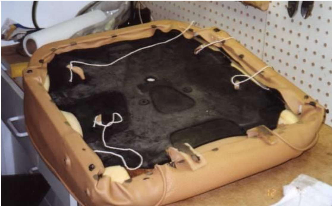
Figure 6 Installing the center pad.
