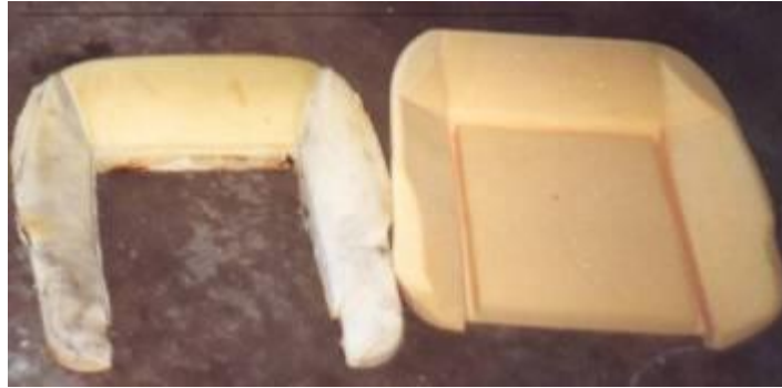
Figure 1 Seat foam, old (left) and new (right)
