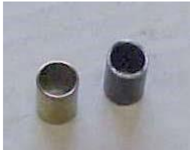
Figure 2 Jaguar and homemade strut spacers.
