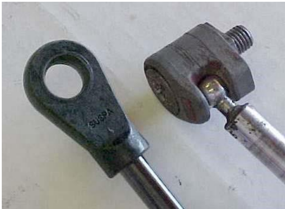
Figure 1 New (left) and old (right) bonnet strut ends
