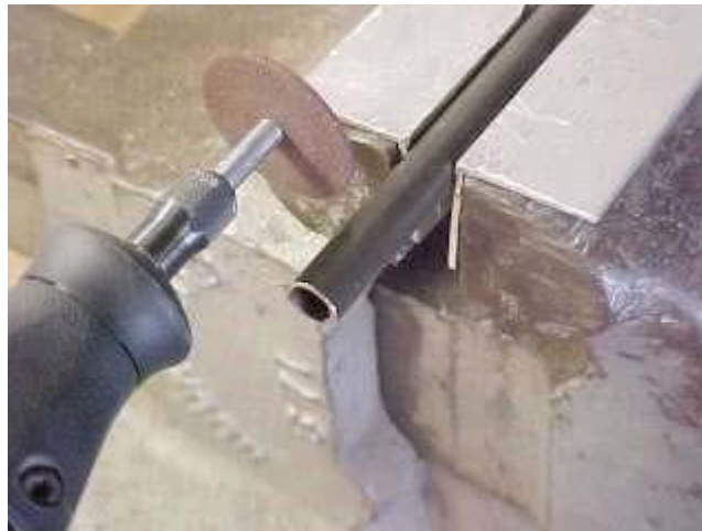
Figure 3 Cutting spacer from brake line.
