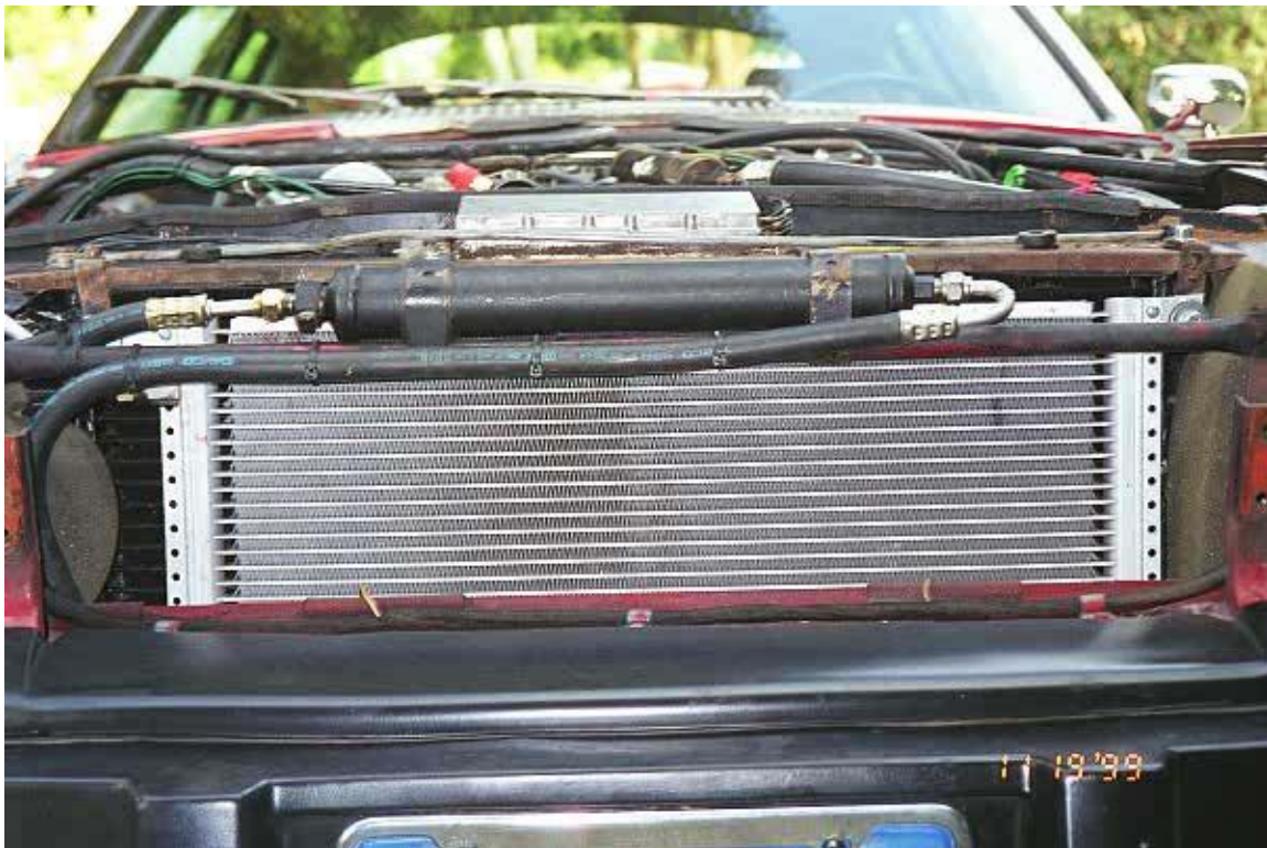
Figure 1. Parallel Flow Condenser installed in 1976 XJ-S.
