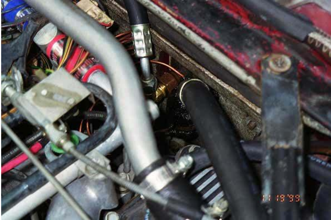
Figure 6. New expansion valve in place (center).
